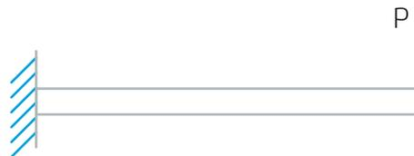
Figure 10. Cantilever beam with a point-applied end load
