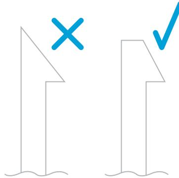
Figure 17. Snap-fit overhang
