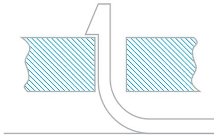
Figure 4. L-shaped snap-fit assembly operation
