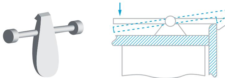
Figure 9. Torsional snap-fit
