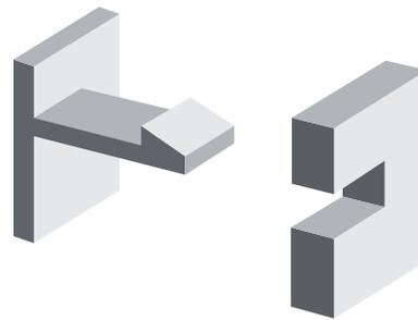
Figure 1. Cantilever snap-fit
