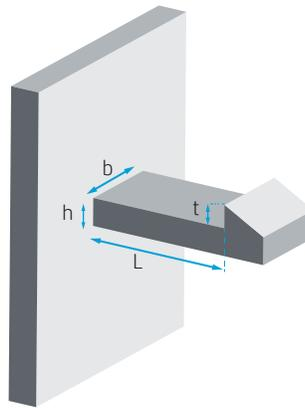
Figure 11. Snap-fit geometry
