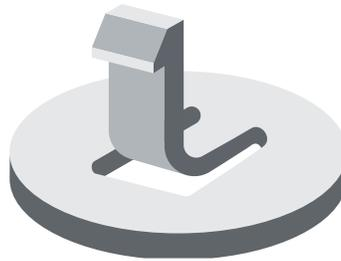
Figure 3. L-shaped snap-fit
